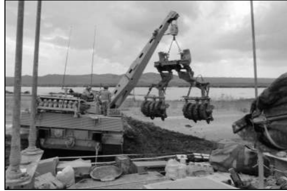
Left: ARV BRUTUS in action under the supervision of the tank-squadron maintenance sergeant. Right: ARV CALGARY recovers T33 mine rollers that had been completely submerged in mud near Sperwan Ghar. (Photos by Capt P. Croteau)
