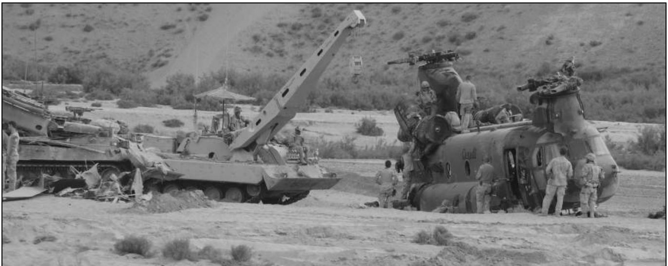
Leopard 2 ARV working on a crashed CH147 Chinook Helicopter (Photo by MWO A. Champagne)
