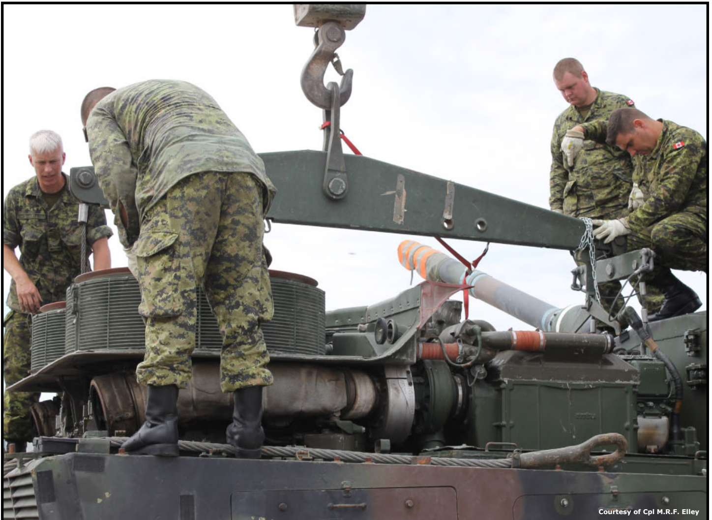
The inaugural Leopard 2A4 CAN D&M courses learning how to replace the pack with the assistance of the ARV.
