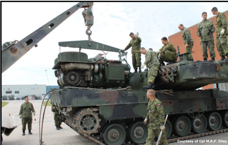
Students on the Leo 2 Instructor Cadre Training learning how to remove the pack. This type of training and standard is now the responsibility of the newly created Army D&M Team.
