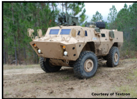
The Tactical Armour Patrol Vehicle (TAPV) Recce Variant will have a crew of four with space for an additional passenger. The armament will be a Kongsberg Remote Weapon Station (RWS) capable of mounting a 7.62mm machine gun and the 40mm Automatic Grenade Launcher. While crew protection was the vital ground for this project, mobility is a key concern for the end user. Of the vehicles competed, the TAPV provided the best overall manoeuvrability.
