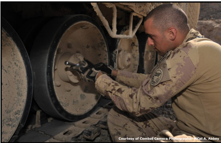
Corporal Fredrick Rodrigue from 12e Régiment Blindé Canada (12 RBC) checks the hub oil on a Leopard 2A6 tank during routine maintenance in Afghanistan
