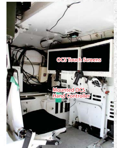
Operator Control Station Main Installations
