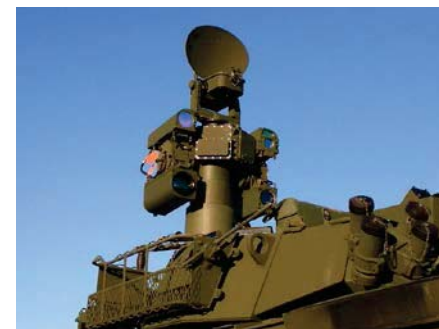
Mast Gimbal with Sensors and MSTAR v6 Radar
