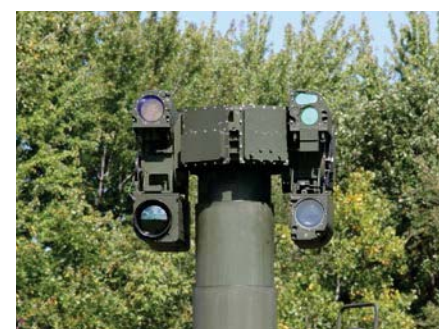
Gimbal and Sensor Pods without MSTAR v6 Radar
