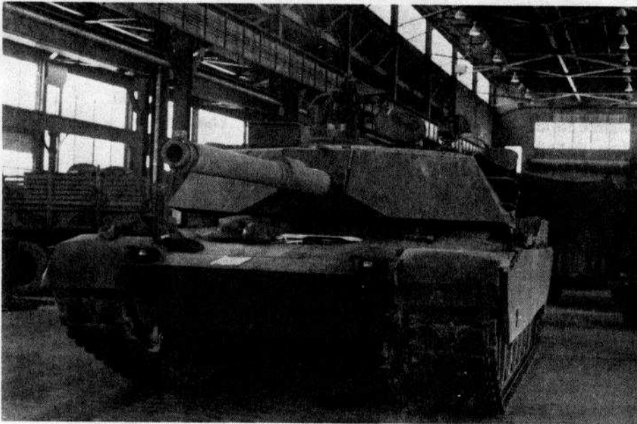
"The XM-1 or General Abrahams tank with its 1500 HP engine and 105 MM gun".
