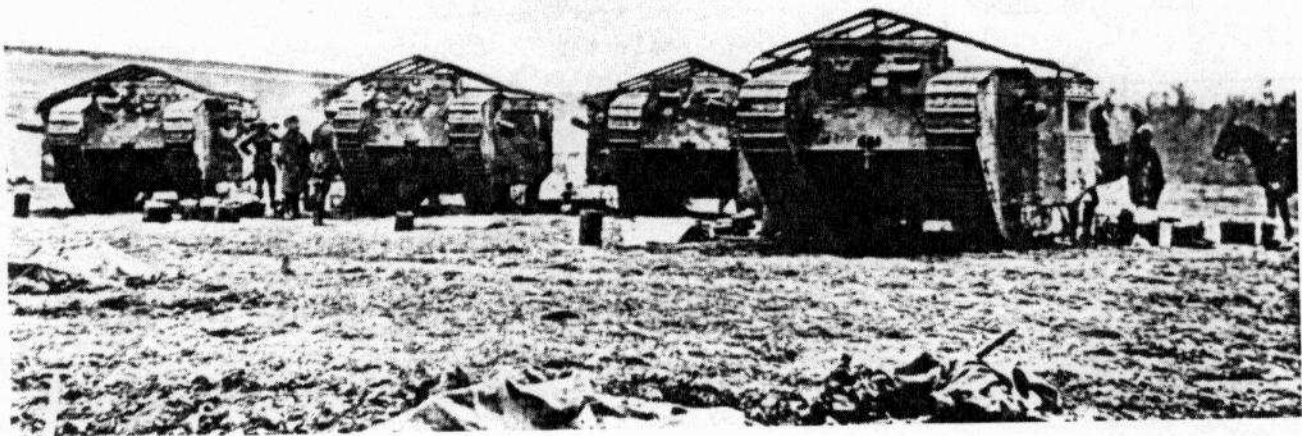
Mark I Tanks preparing for the September debut. Second tank from left is a Male (6 pdr), the others females (MGs). Screen above them was to deflect grenades. Photo courtesy Tank Museum, Bovington.
