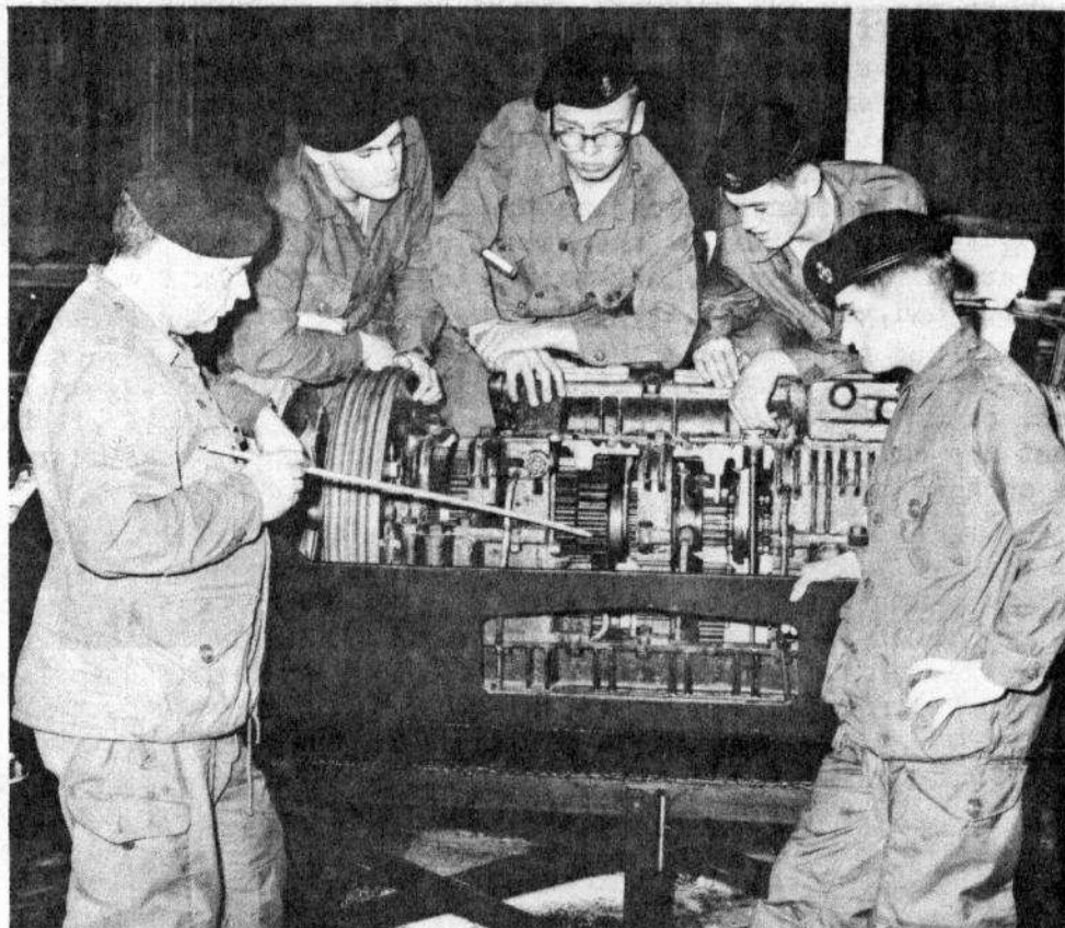
Sgt Barsby instructing on the Centurion transmission compartment
