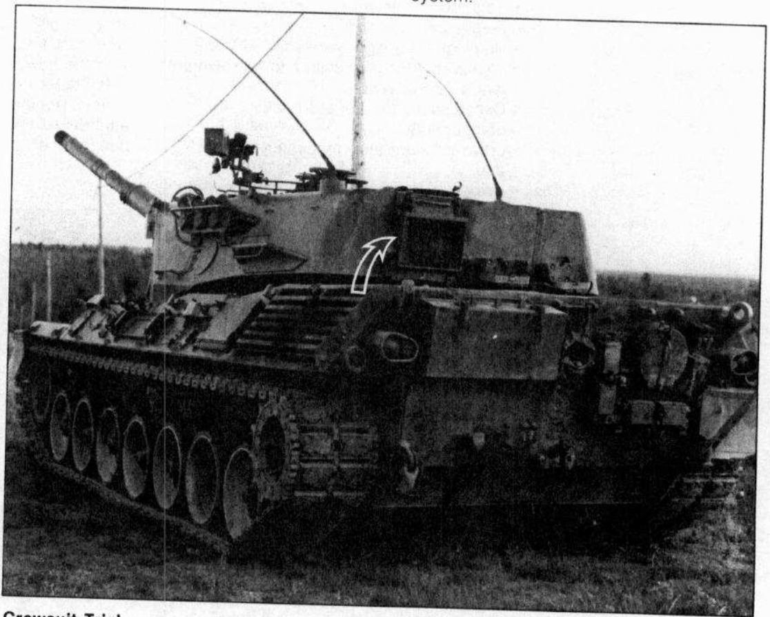
Turret identity light system mounted on the Leopard C1. (CF Photo GNC 89-7364)
