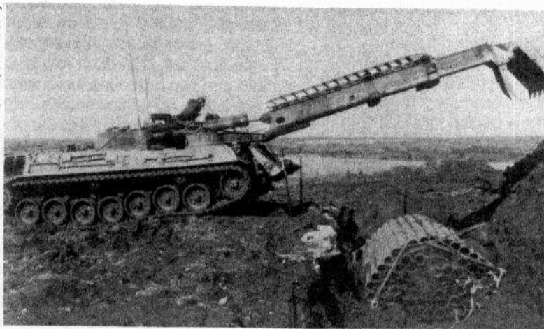
MCpl Bill Kayden of 22 Fd Sqn uses the AEV to drop a fascine into an anti-tank ditch.
