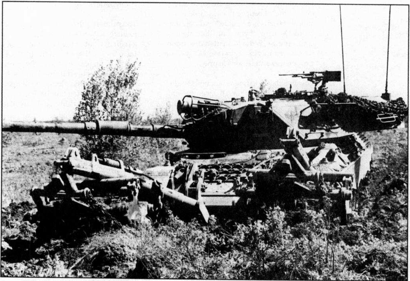
Leopard equipped with track width mine rollers. Is it worth it?
