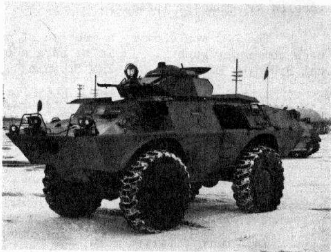
Commando with One-Man One-Meter Turret. .50 cal HMG and 7.62mm Browning GPMG are both mounted.
