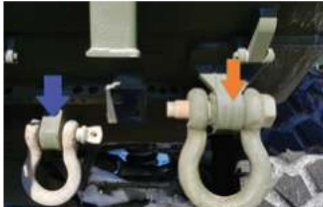
Figure 5 - TAPV Towing U-Hook location (blue) / TAPV Tie-Down Delivery Issued U-Hook (red)
