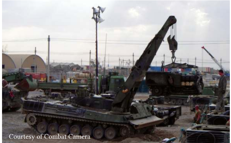
Leo 1 ARV lifting a power-pack in Afghanistan.
