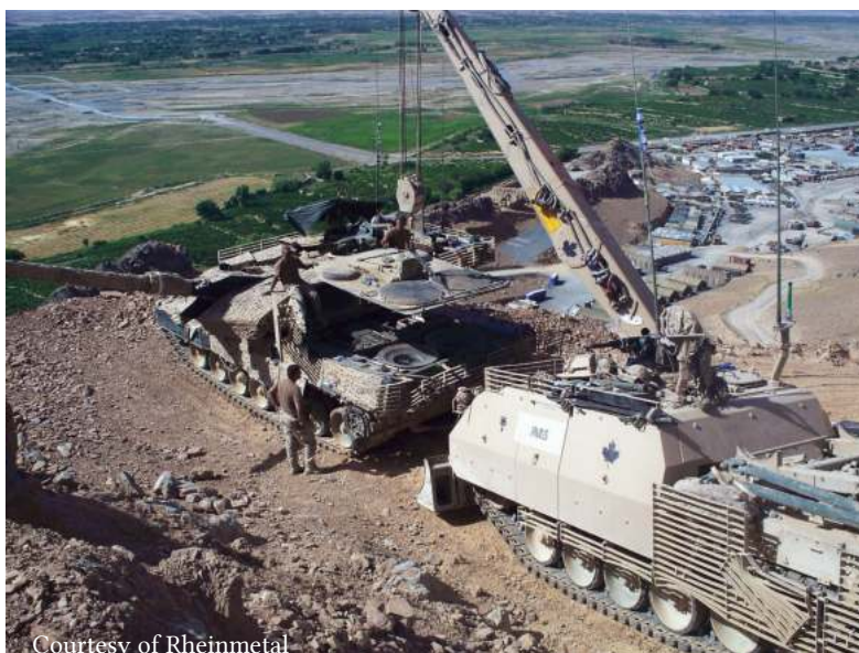
Leopard 2 ARV supporting maintenance on a Leopard 2 power pack in a Forward Operating Base in Afghanistan.
