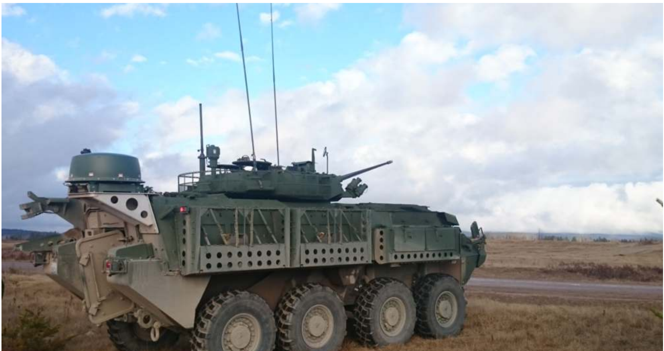
Prototype installation of the SOTM antenna on a LAV 6.0
