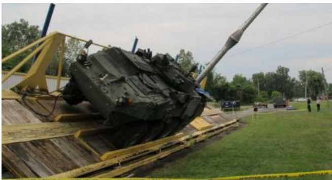
The LRSS Risk Reduction Unit (RRU) with a 10m surrogate mast being tested on a tilt-table at NRC for the Stability/Mobility testing in Definition Phase.
