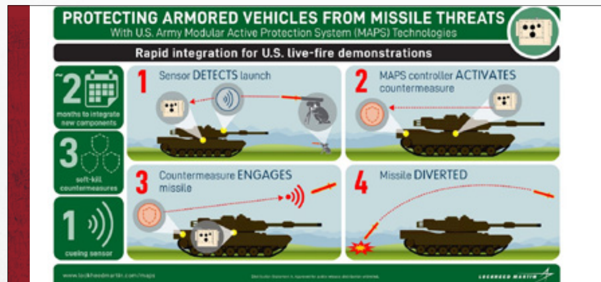
The US Modular Active Protection System overview. Credit: Open source, Lockheed Martin website.
